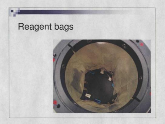
Reagent, standards and waste bags are installed in the lower section of the guard around the outside of the lower housing of the analyzer. The picture shows the view looking in from the top of the lower guard section. Each bag has a specific position in the carousel. Each reagent bag connects to a specific port on the valve.
